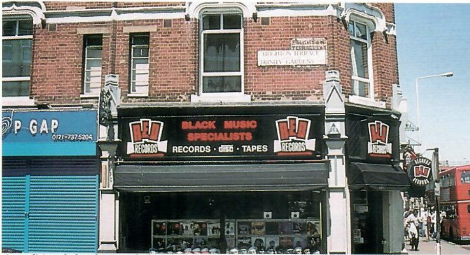
A traditional shopfront including fascia, stallriser and solid pilaster with capitals
