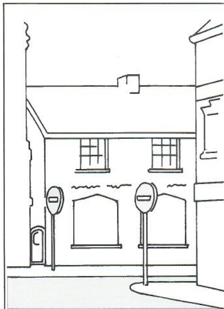
Typical double 'no entry' signs
