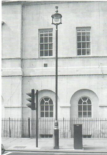
Separate traffic signal and lamp column
