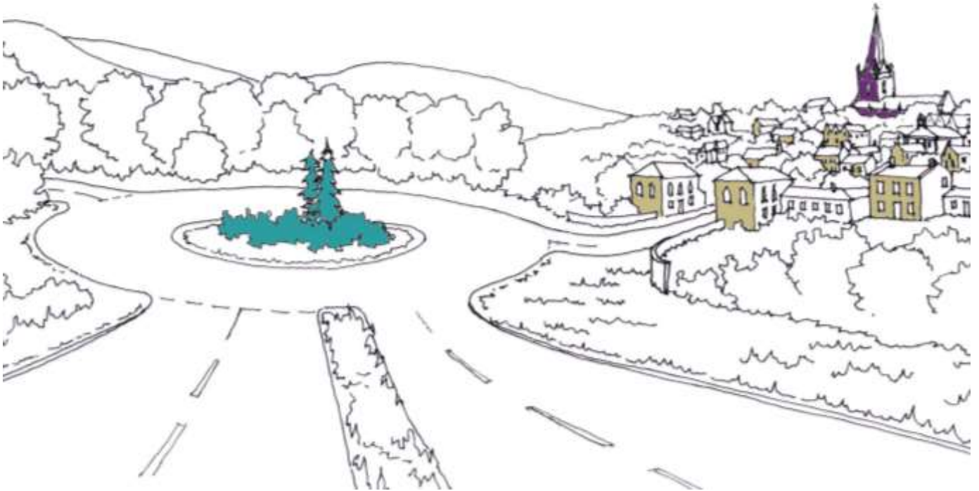
3.15 Regardless of traffic signs, drivers tend to adjust their driving behaviour and speed to what they feel is safe, be it a wide, clear road across open country or a congested road in a town
