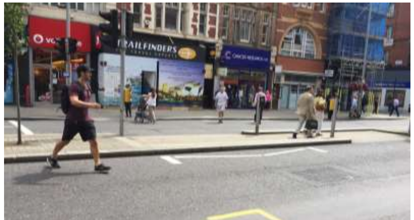
8.05 Guard railing was removed at the reconstructed two-stage crossings
