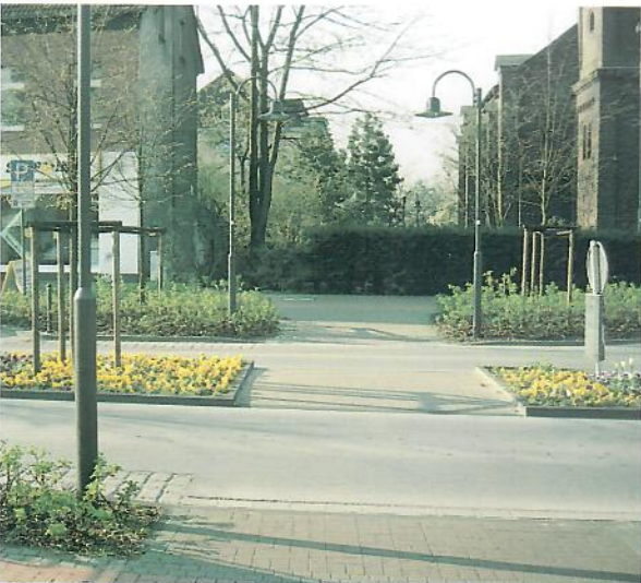
Precise symmetrical layout at a pedestrian crossing combined with a carriageway narrowing
