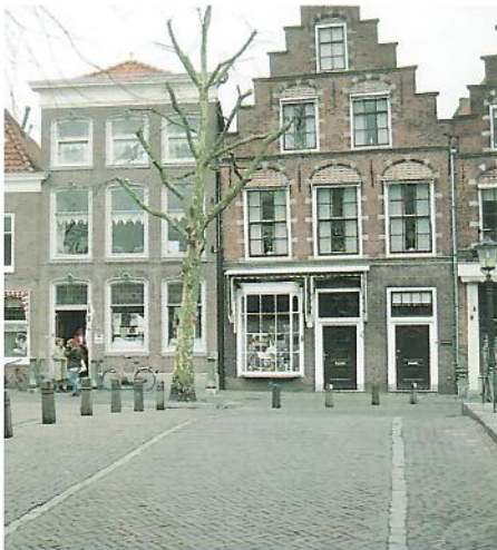
Surface for vehicles indicated by a subtle texture change and equally spaced bollards
