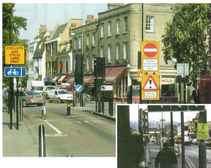
Less is more: Bus gate (above) and typical clutter outside a town centre (inset)
