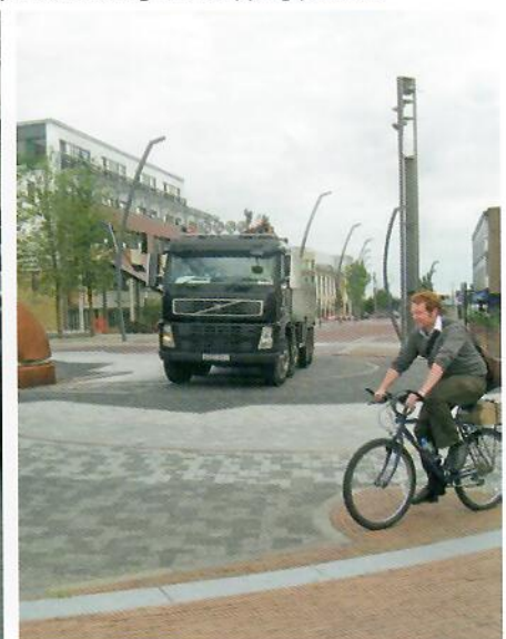
Roundabout with all signs removed
