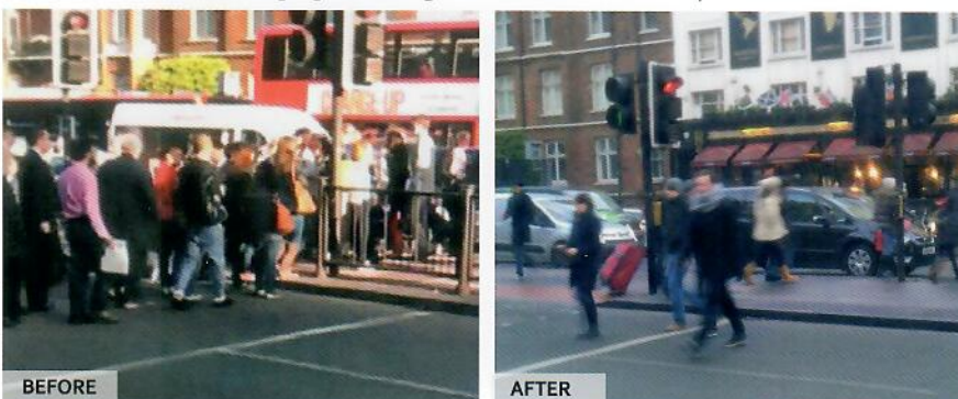
Guardrailing forces pedestrians into a narrow area where they may be trapped in the road
